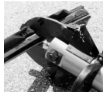
The proper way to cut. The blades are perpendicular to the piece being cut.
