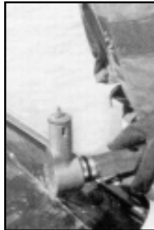
Strike windshield with top of tool to make puncture point.
